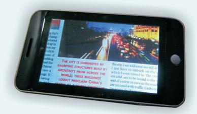
The handheld unit is used to capture images when the user is on the move and can be docked to a custom desktop with HDMI display to provide magnification
