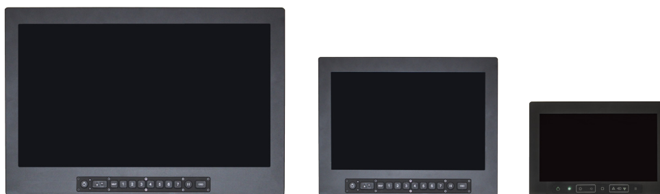
Figure 2: Members of the new Curtiss-Wright SVDU rugged mission display family (left to right: 21.5" SVDU5500, 14.1" SVDU3600, 7" SVDU1800)
