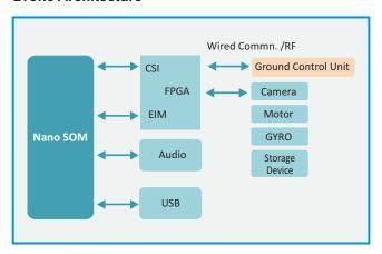
For this application, we can design a custom board for the Drone using a FPGA to implement the logic for taking in the multiple camera & sensor inputs, required for self-navigation; formatting the data and sending the same to the Nano SOM. The Audio functionality is implemented to capture and transfer the data to ground system.
