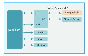
We can also design a custom board for the ground control system using a FPGA to implement the logic for acquiring the streamed camera data and formatting the same to be sent to the Nano SOM camera port.
