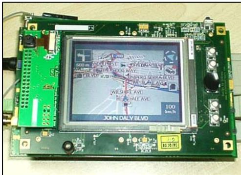
The Navigation Reference Design supports SmartST™, navigation software from Navman and has four RF modules: GPS, GSM/GPRS, WLAN and BLUETOOTH on a single small form factor board running Microsoft Windows® CE on TI's OMAP5912 processor. The NRD provides product developers with an easy-to-use platform to simulate or test their GPS and wireless applications. This reference design can
