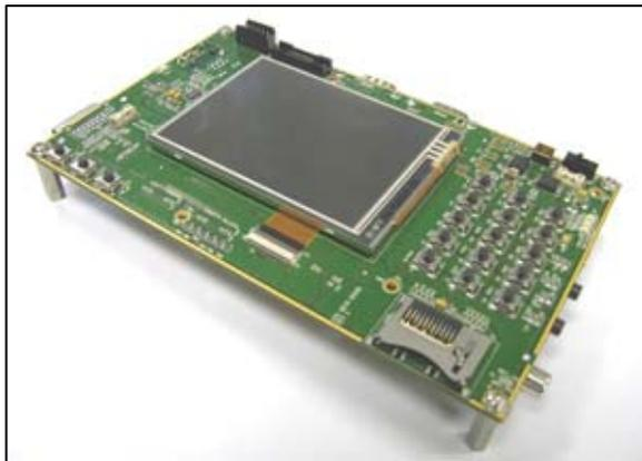
The OSK is designed with a modular and extendable architecture. It is comprised of separate processor and power modules providing reconfiguring flexibility to future processors and power modules. Expansion connectors on the board provide extensibility to a wide range of peripheral interfaces. A key feature of the OSK is the support for an LCD display and DVI to connect to external digital display devices.
