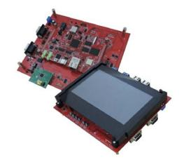
The AM437x PoM and Application Board comes integrated with U-Boot, Linux SDK (3.12), Android Kitkat (4.4.4) and demo applications. The PoM and Application Board can be used to build Video Door Phones, Control Panel, Industrial HMI and PLC, Barcode scanners, Portable Data Terminals, Non-invasive Medical Electronics and Assistive technology products.
