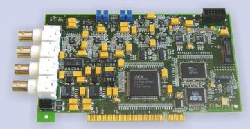
This Case Study showcases a PC based high-speed recording solution designed by Mistral featuring 4-channels 14-bit data conversion resolution, up to 128X speeds with Windows based GUI.
