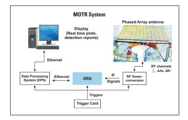
The following list enumerates the functions of the DRS, which are typical of RADAR receivers.
