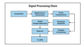
In order to meet the stringent processing requirements, Mistral recommended a COTS VPX based Hybrid computing platform with a Dual Core PowerPC processor and two Xilinx Virtex-6 SX series FPGAs. The FPGAs are used for accelerating the signal processing and detection algorithms. All processing was done using IEEE-754 single precision floating point arithmetic.
