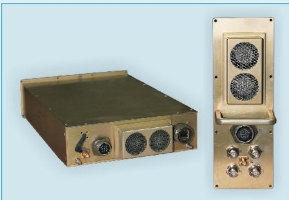
“ The V/UHF Wideband and Microwave Receiver is a signal interception, analysis and monitoring receiver subsystem ”
