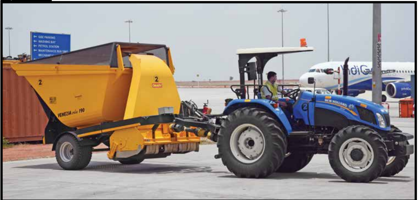
↓ Driven by a 90 hp Holland tractor, a grass maintenance machine from Italy trims lawns.
