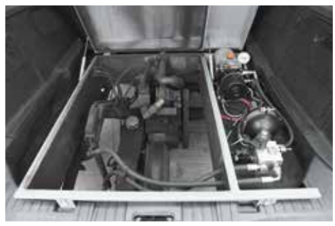
↑ A Ford Galaxy estate procured from Sweden as an AIRPORT SURFACE FRICTION TESTER (ASFT) measures friction on airport runways and taxiways with the help of a measuring wheel at the rear.
