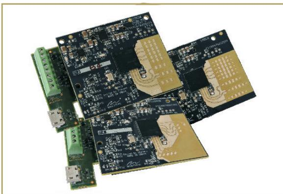
The Automotive RoM operates at frequency bands of 76-81GHz & is ideal for next gen ADAS applications.
