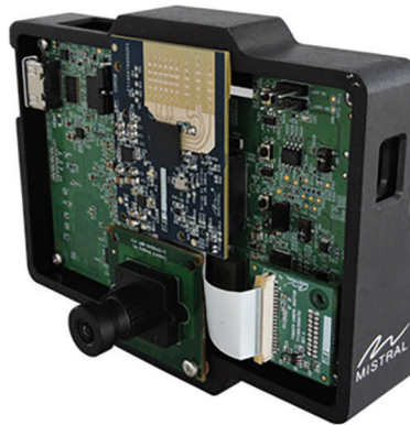
An integrated, camera and mmWave radar sensor platform based on Texas Instruments TDA3 SoC and AWR1443 FMCW RADAR sensor for ADAS applications.
