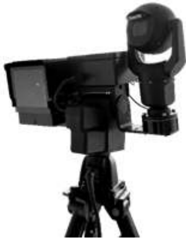
Figure 5: EO Sensor for Drone Detection
