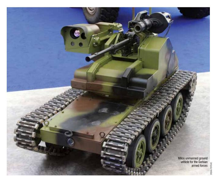
breaking, and so on. An electric platform also brings in advantages like minimal heat signature, low noise, lesser vibration and relatively less weight. A UGV platform designed or chosen for defence applications need to support at least a 500kg payload, in addition to the weight of all electronics and sensors integrated into the system, considering the typical applications like emergency evacuation, payload/arm delivery, etc.
