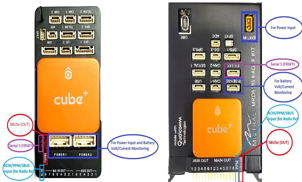
Figure 1: Pixhawk-Base & Eagle Kit power / telemetry interfaces
