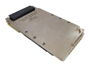
Engineered for applications demanding exceptional compute power and advanced signal processing, the VPX3U-AGRW014 integrates the Agilex 9 FPGA, and Cortex A53 Quad Core ARM with high-performance wideband data converters for superior fidelity and robust processing capabilities. The card's architecture leverages Intel 10 nm SuperFin technology to achieve a high channel density with transceiver rates up to 58 Gbps, ensuring ultra-low latency and exceptional data throughput.
